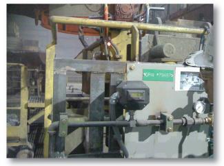
Thermal mass flowmeters are commonly used to measure argon during steel production. However, these meters require frequent recalibrations in order to maintain optimal performance. Thermal mass flowmeters are also less accurate than precision flow instruments such as turbine meters.
