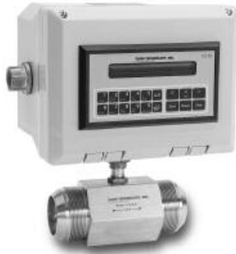
The FC70A-B1-A6 is shown mounted directly on a Flow Technology 2-inch turbine flowmeter. The FC70A is housed in a NEMA 4X/IP65/Exn enclosure with two conduit hubs. The enclosure is also available with MS connectors for cable connections. The FC70A panel mount configuration has a watertight seal which meets NEMA 4X/IP65 standards.
