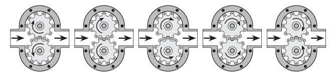
Flow Technology positive displacement flowmeters use two rotating impellers driven by the flowing liquid. Magnets imbedded in the impellers activate a non-intrusive sensor which generates a pulsed output signal. Each pulse represents a known volume of liquid that is captured between the lobes of the impellers. A K-factor converts the pulses into engineering units for remote data collection and digital display.
