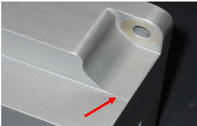
Unacceptable Machined Step
