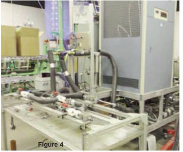
was flowed through the meters corresponding to approximately 41 days of continuous operation. It should be noted that these meters were run at ~90% of their flow range (i.e. at high speed) and due to the heating effect of the pumps water circulated at approximately 70°C. These factors will have a tendency to accelerate bearing aging reducing the life expectancy of the bearings. Figure 5 details the shift in K-factor for both units over the evaluation period.
