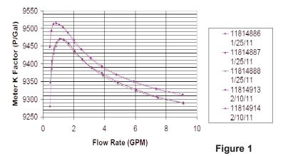
K-Factor curve is typically an indicator of bearing wear. The graph in figure 1 details the performance of Manufacture C's unit after 1 week of operation; as can be seen significant calibration shifts can already be observed! Manufacture C's unit failed after 12 days of continuous operation: The bearings wore out, physically disintegrating.
