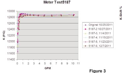
The meters were then installed in a recirculation water loop at ~7.5 GPM (see Figure 4) and were periodically removed to perform a calibration check. Approximately 450,000 gallons of water
