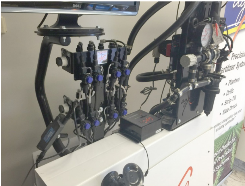
QCT Series in-line ultrasonic meter on tractor-mounted spray system
