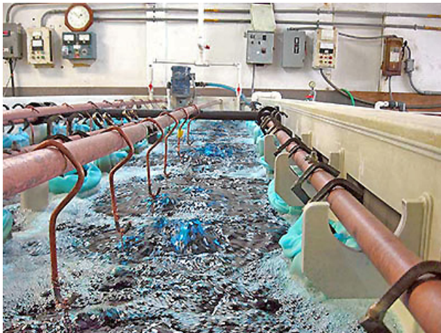
Plating tank with automatic part dipping system
