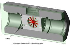
Sometimes referred to as a Pelton Wheel or Paddle Wheel design, this design is generally considered to be the best solution for efficient conversion of flow energy.
