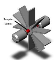
rotor is pressed onto the shaft and the shaft rides in a sapphire pivot vee pressed into the set screw assembly. A spring is incorporated into one side of the set screw assembly to maintain a constant force on the shaft.
