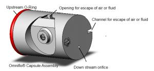
Fluid flows through the orifice, impinges on the perpendicular rotor blade and most fluid exits through the downstream orifice. Residual fluid and any air or other gaseous substance existing in the line can escape the flow meter from an opening in the top of the Omniflo® and a channel machined into the capsule assembly.
