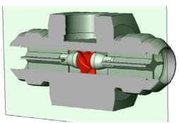
to spin in proportion to the volumetric flow through the flow meter.
