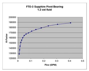
The Omniflo® flow meter is repeatable to +/-0.1% reading over the normal flow range of the flow meter, with a non-linear output over the entire flow range. This is due to the low kinetic energy of the low flow applications and necessary mechanical conversion of that energy. Although the most efficient designs are applied, friction overcomes the available energy, resulting in a non-linear output.
